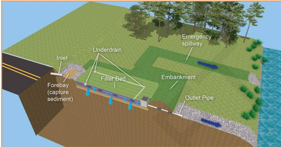
**Figure 5.5-2 Typical Surface Sand Filter Configuration and Components**
