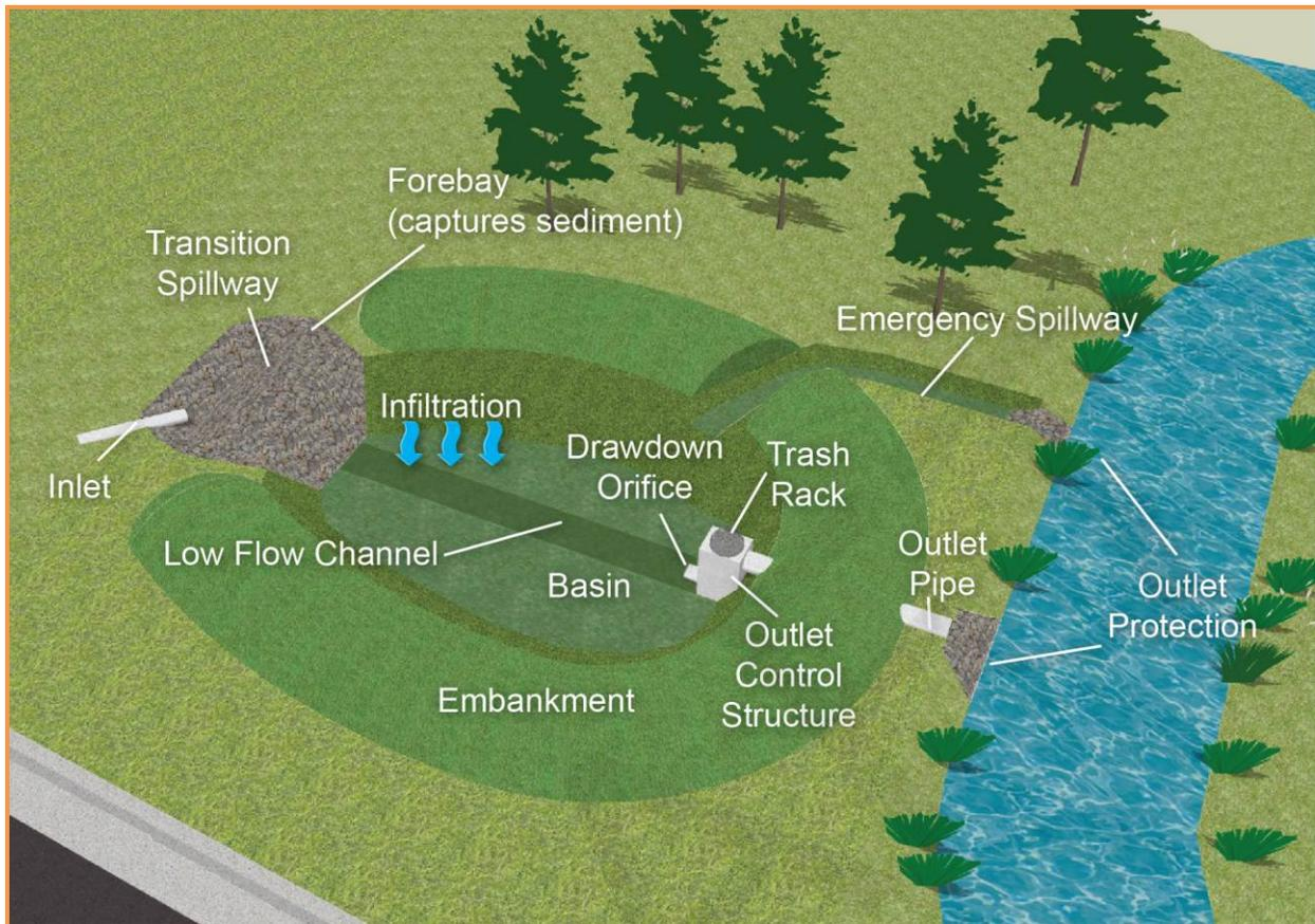
**Figure 5.6-2 Typical Dry Detention Basin Configuration and Components**
