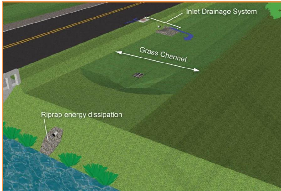
**Figure 5.2-2 Typical Grass Channel Configuration and Components**
