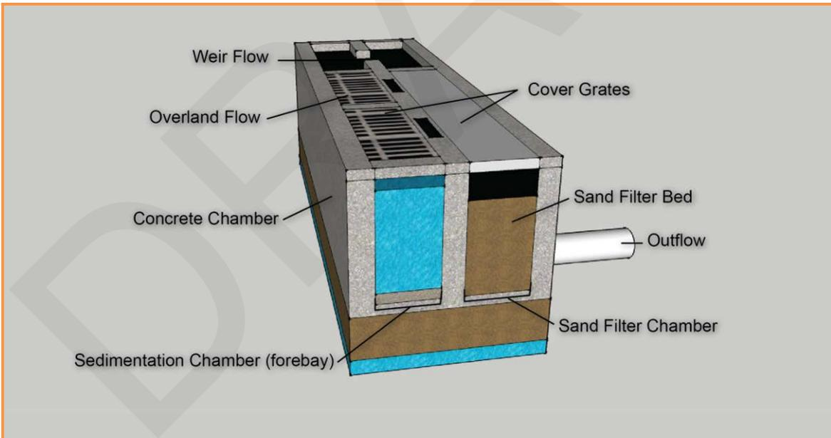
**Figure 5.5-3 Typical Perimeter Sand Filter Configuration and Components**
