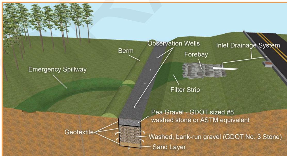
**Figure 5.4-1 Typical Infiltration Trench Configuration and Components**
