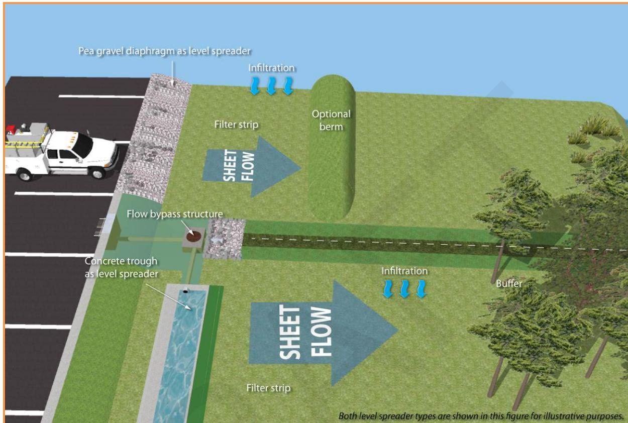
**Figure 5.1-2 Typical Filter Strip Configuration and Components**
